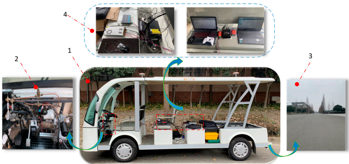
Figure 11. A test LSEV equipped with HMRBS. 1—Sightseeing vehicle; 2—HMRBS; 3—Test road; 4—High precision GPS/IMU system and CAN data analyser.
