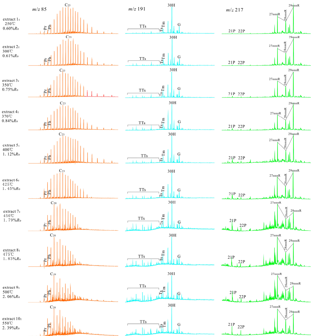
Figure 5. The m/z 85, m/z 191 and m/z 217 mass chromatograms showing the distribution of the saturated hydrocarbons ( n -alkanes, terpanes and steranes, respectively) from the extracts of solid residues. Note: Pr = Pristane, Ph = Phytane, TTs = tricyclic terpanes; Ts = C 27 18 \alpha (H)-22,29,30-trisnorhopane, Tm = C 27 17 \alpha (H)-22,29,30-trisnorhopane, 30H = C 30 17 \alpha (H), 21 \beta (H) hopane, G = Gammacerane, 21P = C 21 aaa pregnane, 22P = C 22 aaa methylpregnane, 27aaaR = C 27 aaa 20R stigmastane, 28aaaR = C 28 aaa 20R stigmastane, 29aaaR = C 29 aaa 20R stigmastane.
