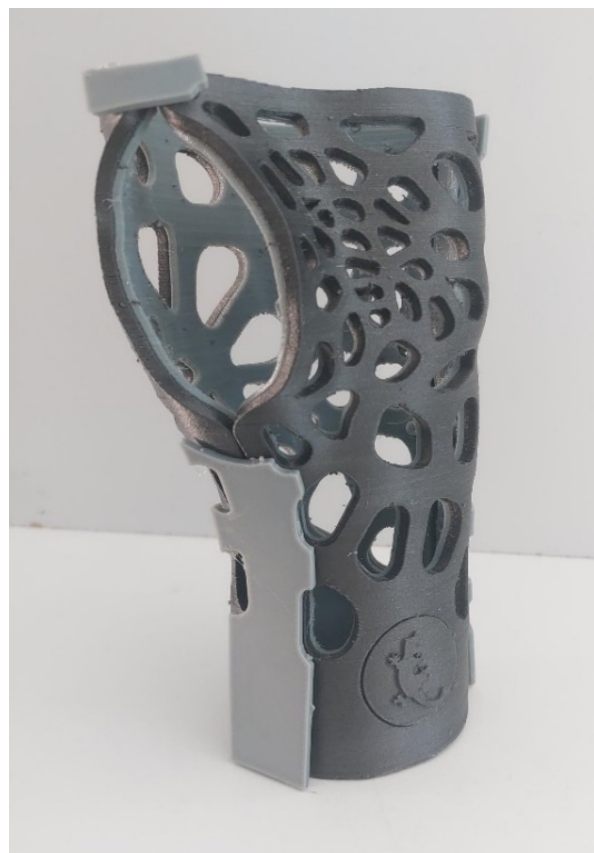
Figure 23. The fabricated developed WHO.
