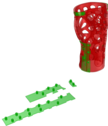
Figure 10. Formation of 3D bands with fastening mechanisms and unrolling: (a) wavy joints; (b) unrolling of the three bands.
