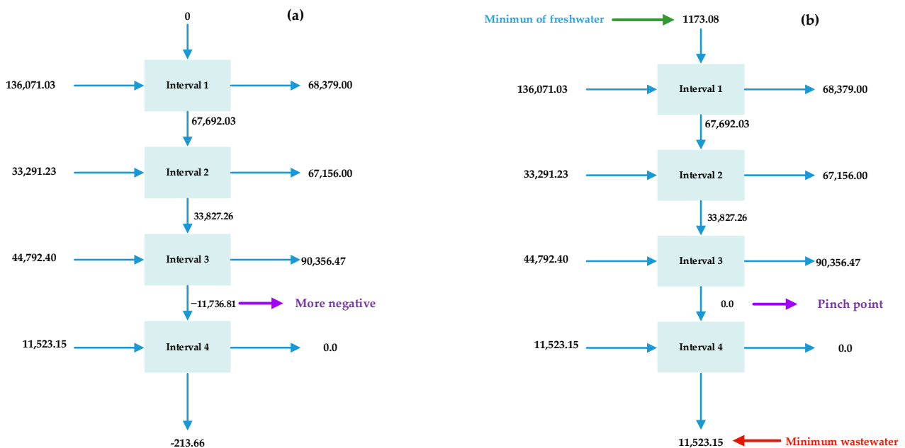
Figure 6. Cascade diagrams for Category 1 at (a) Base case and (b) mass-integrated topology.
