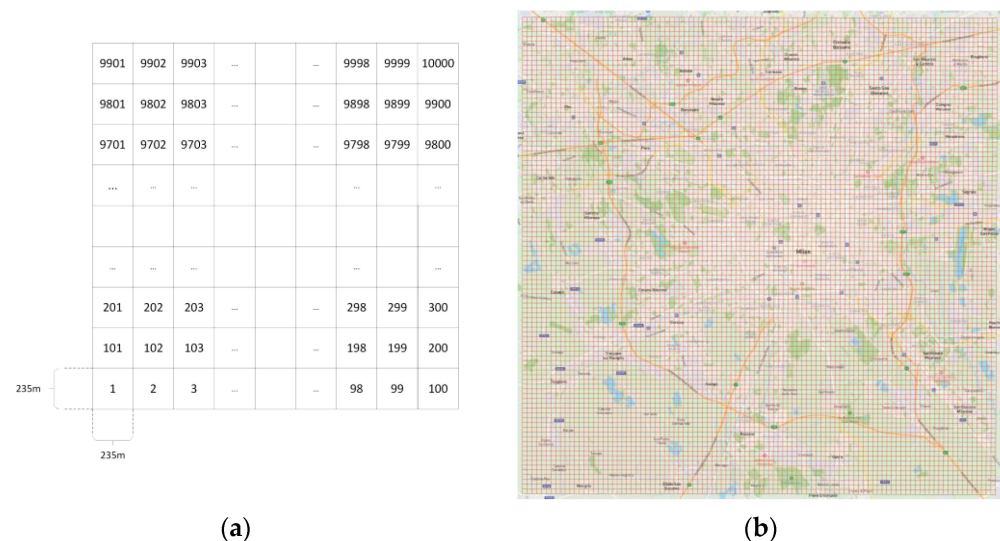
Figure 1. The Basic information of Milan grid division: (a) the grid ID identification and the method of Milan grid division; (b) the specific situation of Milan grid division.
