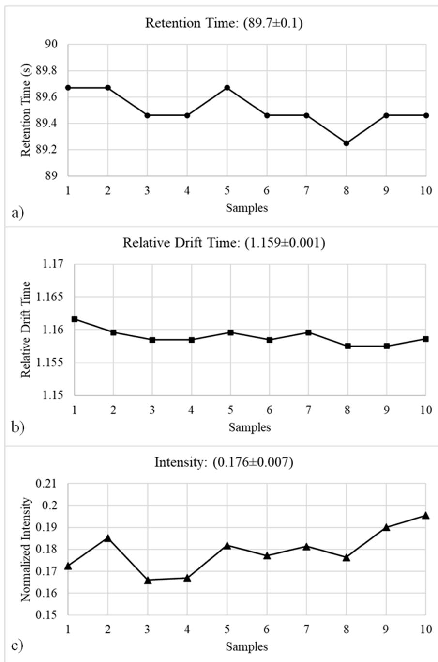
**Figure 4.** Repeatability graph for the retention time (a), the relative drift time (b), and the normalized intensity (c) for ten samples of a randomly selected analyte (dimer of acetone) analyzed with the GC-IMS.
