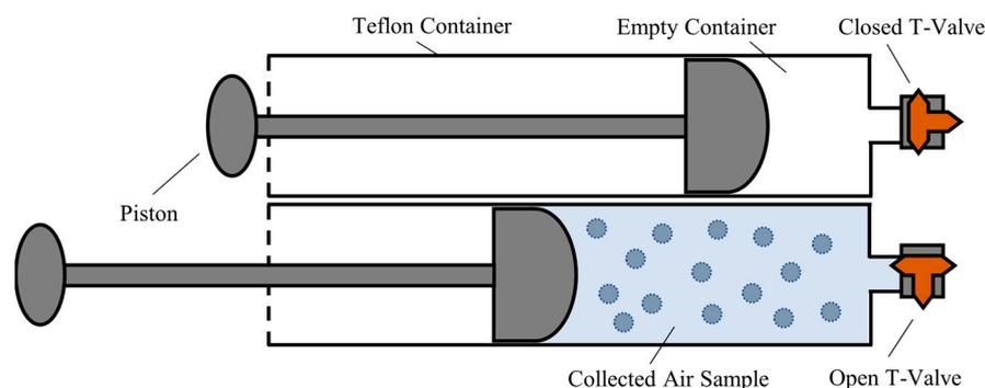
**Figure 3.** Procedure for collecting the air samples with a Teflon container.
