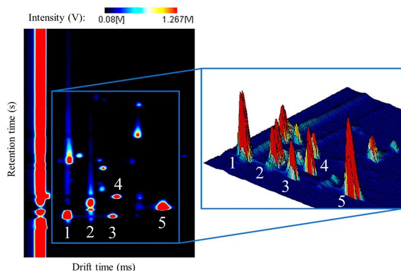
**Figure 2.** Example of a three-dimensional spectrum produced after an IMS analysis, in which some VOCs are identified for elucidative purposes (1—monomer of ethanol, 2—monomer of 2-propanol, 3—dimer of ethanol, 4—monomer of acetone, and 5—dimer of 2-propanol).
