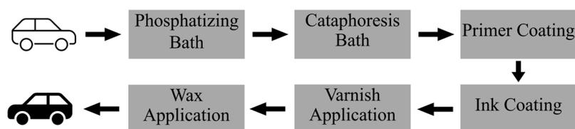
**Figure 1.** Main steps of the coating process in a car factory painting line.
