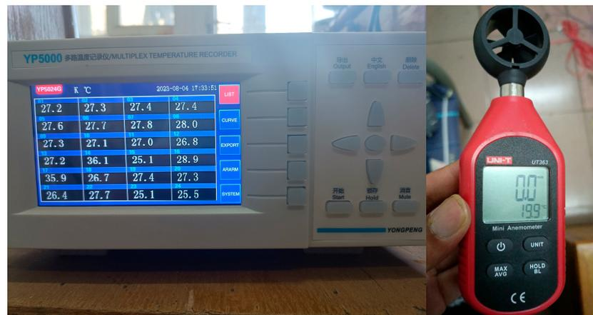
**Figure 5.** YP5000 multi-channel temperature recorder and anemometer.
