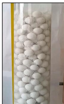
Figure 2. Photograph of the alumina balls ( $\alpha$ -Al<sub>2</sub>O<sub>3</sub>) packing material in the BCR.
