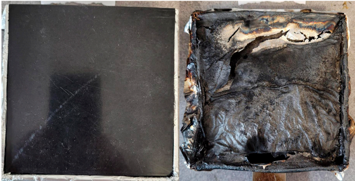
Figure 9. Photo of a polyurea–polyurethane coating with the addition of 10% RDP and 5% TCPP, before and after combustion.
