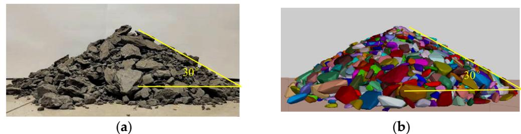
**Figure 2.** Physical and numerical natural repose angle test results: (a) Physical test; (b) Numerical test.
