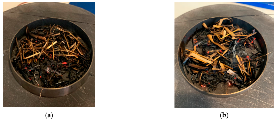
Figure 4. Samples after ignition: (a) 2 g of hay sample, measurement at 1020 s; (b) 2 g of straw sample, measurement at 1050 s.
