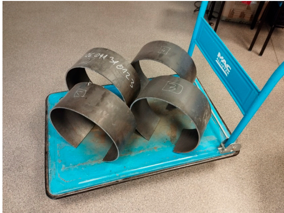
Figure 7. Pipe samples after sectioning for metallographic test.
