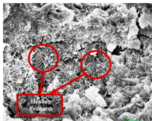
Figure 18. Microstructure of the HUN3 concrete after 14 d of self-healing (180 dry–wet cycles) [4,85].
