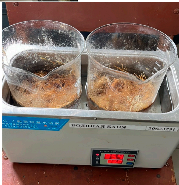
Figure S2. Boiling straw in a water bath.
