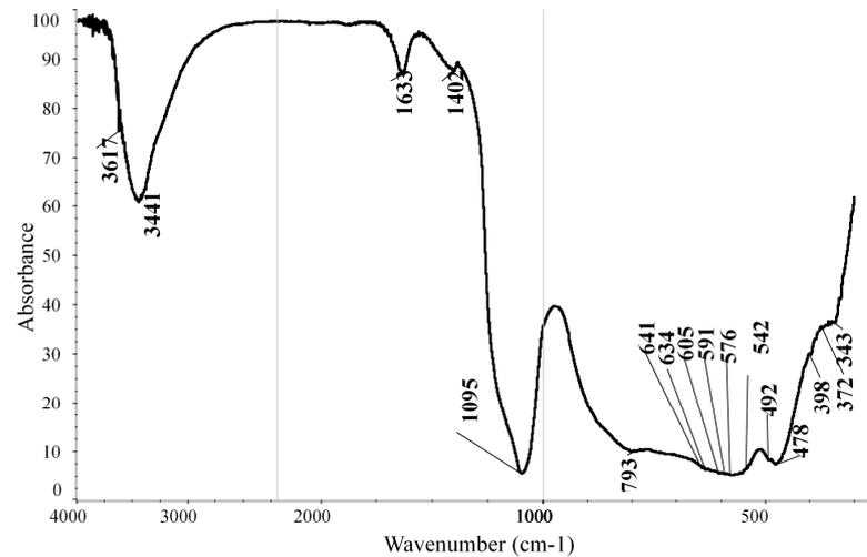
**Figure 10.** Infrared spectrum of the FKF after sintering at  $950\text{ }^\circ\text{C}$ .
