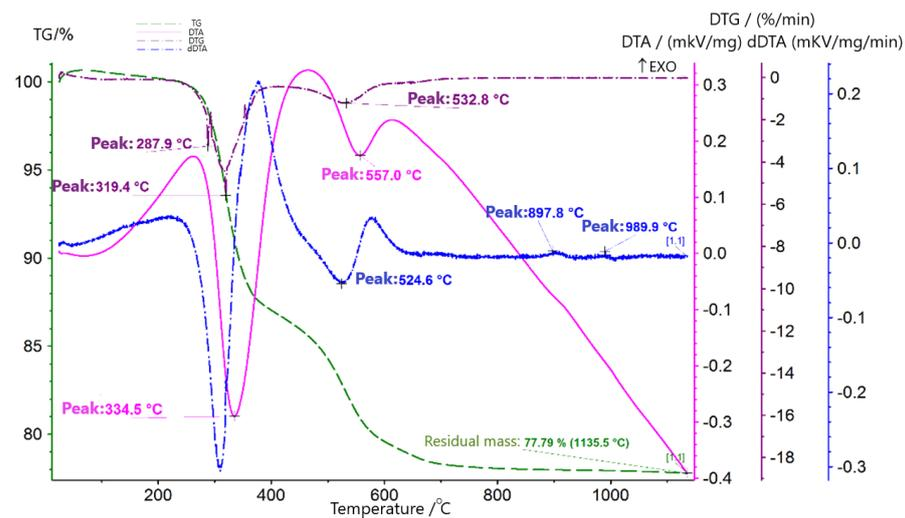
Figure 3. Thermogram of the initial gibbsite-kaolinite bauxite sample from the Krasnogorsk deposit.
