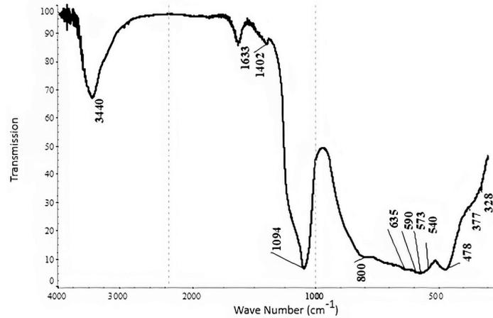
**Figure 9.** Infrared spectrum of the FKF after sintering at  $900\text{ }^\circ\text{C}$ .
