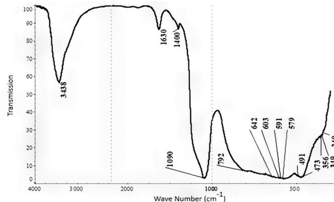
**Figure 11.** Infrared spectrum of the FKF after sintering at  $1000\text{ }^\circ\text{C}$ .
