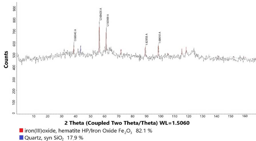
Figure 7. X-Ray image of the FKF after sintering at 950 °C.
