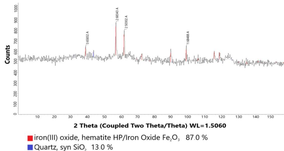
Figure 8. X-Ray image of the FKF after sintering at 1000 °C.
