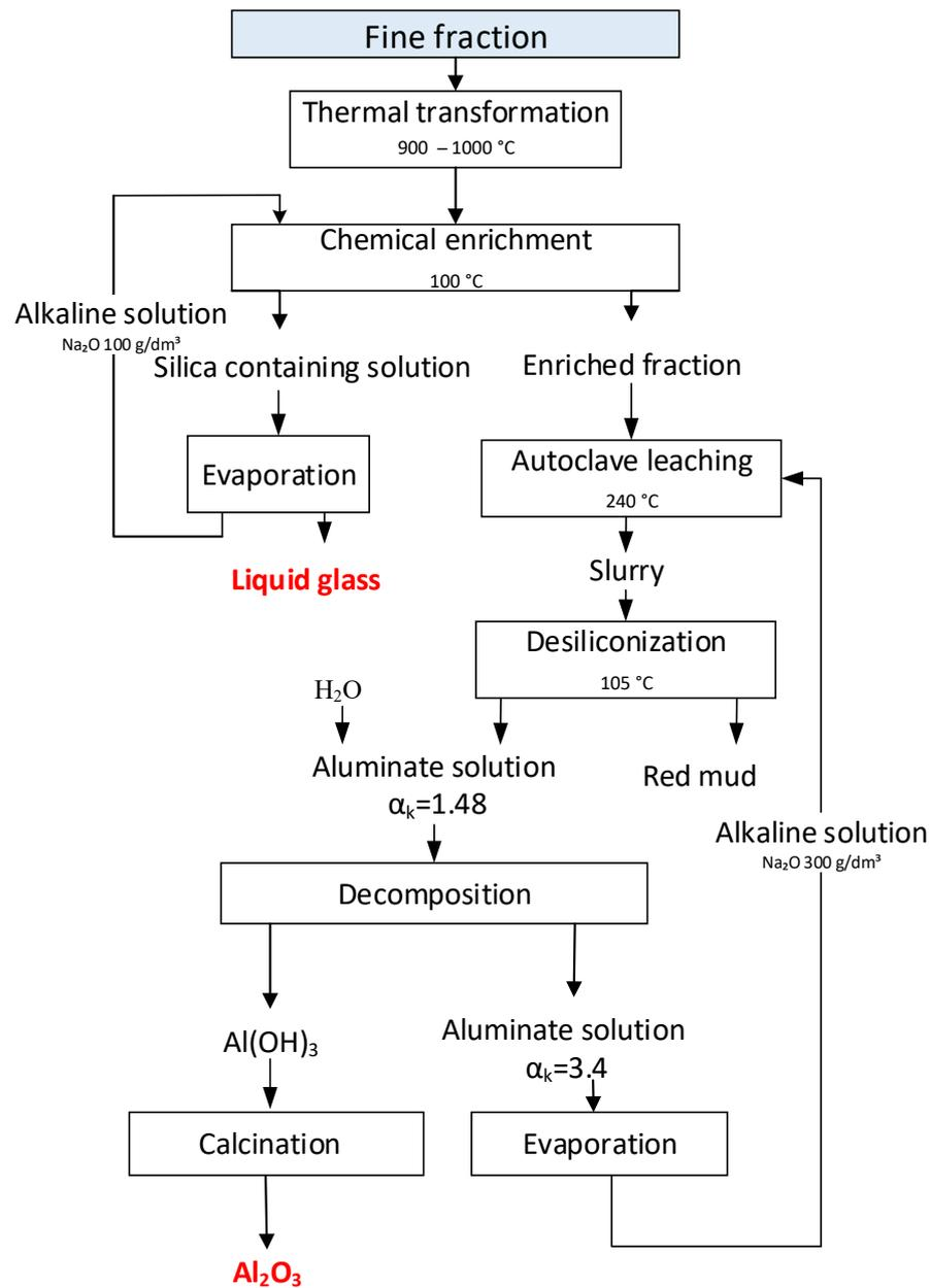
**Figure 4.** Technological scheme for processing the FKF.
