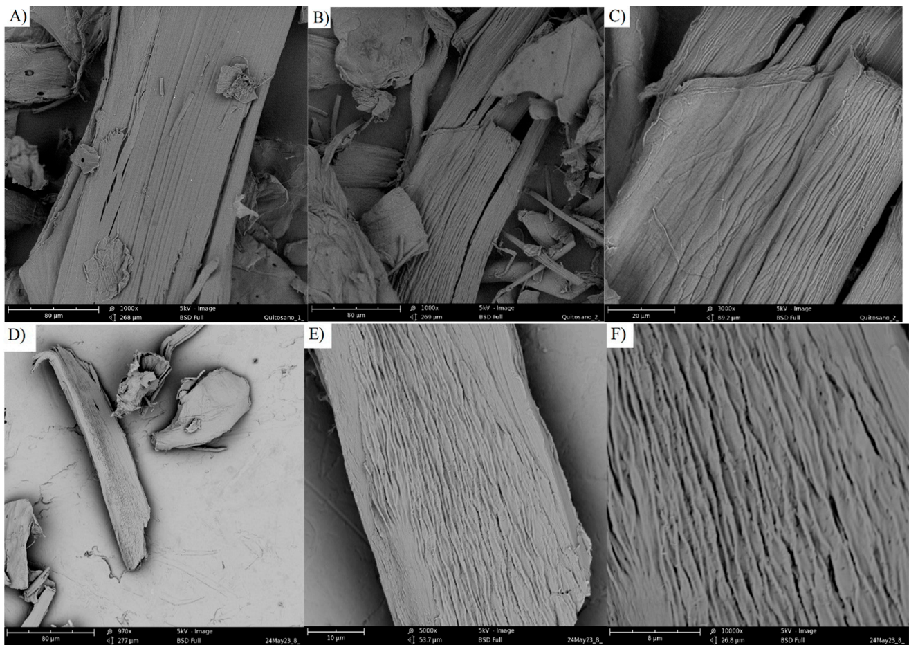
Figure 5. SEM images of chitin extracted from Acheta domestica cricket flour (upper row) with a 970x (A), 5000x (B), and 10,000x (C) close-up and of chitosan extracted from Acheta domestica cricket flour (lower row) with a 1000x (D,E) and 3000x (F) close-up.
