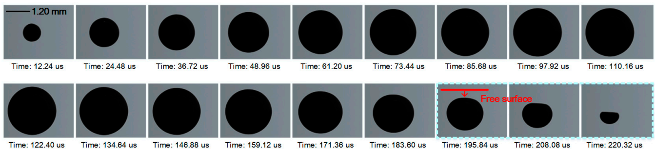
Figure 3. Cavitation bubble dynamics near the free surface. Time: 0–110.16 \mu\text{s} , the expanding cavitation bubble. Time: 122.40–220.32 \mu\text{s} , the contracting cavitation bubble, and apparent non-spherical deformation, r_f = 1.30 , R_m = 1.20 mm.
