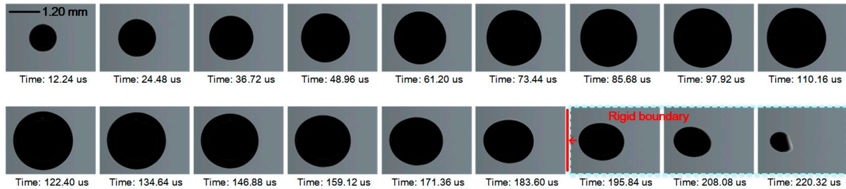
Figure 6. Cavitation bubble dynamics near the rigid boundary. Time: 0–110.16 \mu s, the expanding cavitation bubble. Time: 122.40–220.32 \mu s, the contracting cavitation bubble, and apparent non-spherical deformation, r_b = 1.30 , R_m = 1.20 mm.
