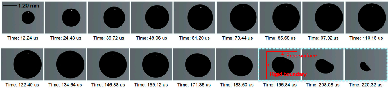
Figure 12. Cavitation bubble dynamics near free surface and rigid boundary. Time: 0–110.16 \mu\text{s} , the expanding cavitation bubble. Time: 122.40–220.32 \mu\text{s} , the contracting cavitation bubble, and apparent non-spherical deformation, r_b = r_f = 1.30 , R_m = 1.20 mm.
