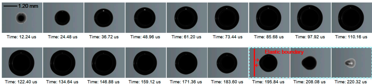
Figure 10. Cavitation bubble dynamics near the elastic boundary. Time: 0–110.16 \mu\text{s} , the expanding cavitation bubble. Time: 122.40–220.32 \mu\text{s} , the contracting cavitation bubble, and apparent non-spherical deformation, r_b = 1.15 , R_m = 1.20 mm.
