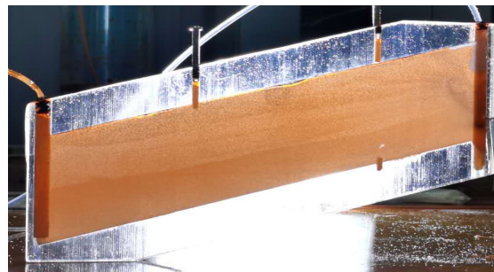
Figure 12. One injection, one production displacement experimental model.
