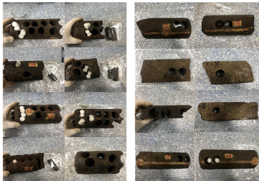
Figure 3. Loose sandstone reservoirs with real core samples.
