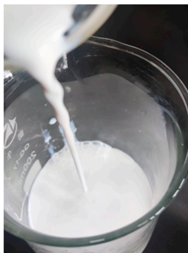
Figure 8. Flow state of latex after repeated freezing and thawing.
