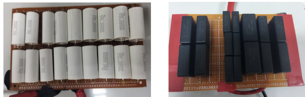
Figure 13. Compensation boards. Ground side (left) and ground side (right).
