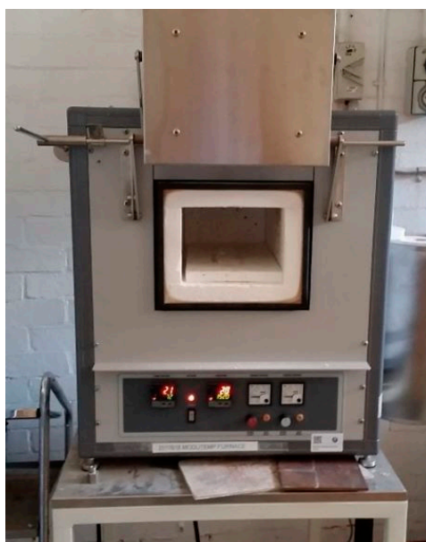
Figure S4. Photograph of the muffle furnace used for the sample pyrolysis.
