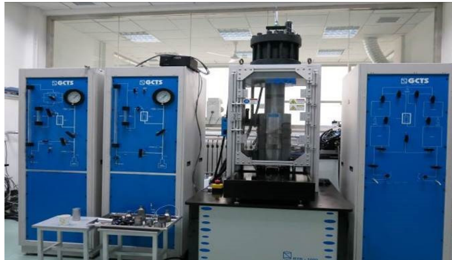
Figure 7. Triaxial testing system by GCTS in the United States.
