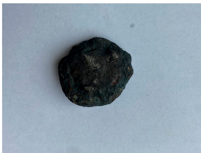
Figure 18. Iron alloy obtained by smelting at 1700 °C.
