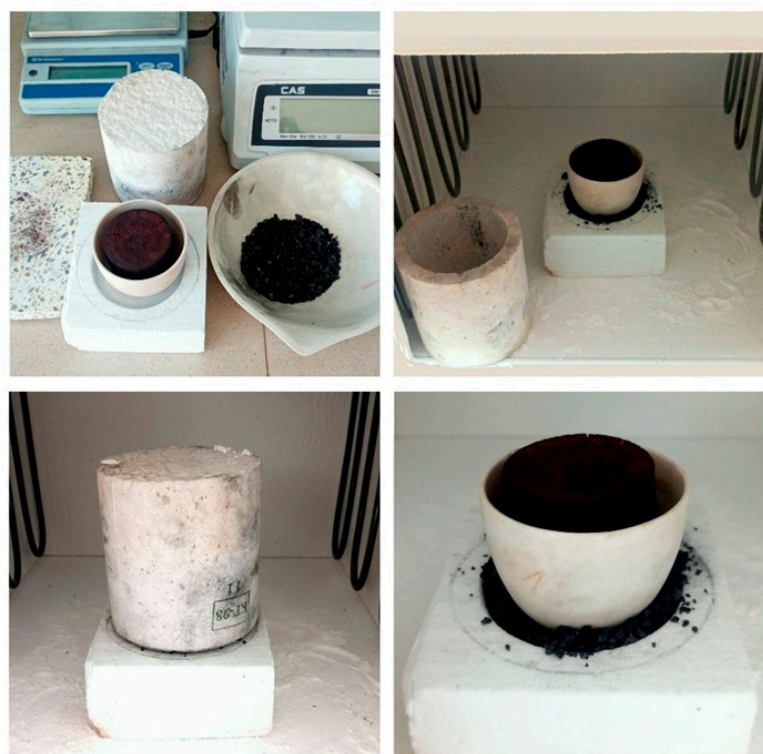
Figure 1. Preparation of briquettes for smelting at 1700 °C.
