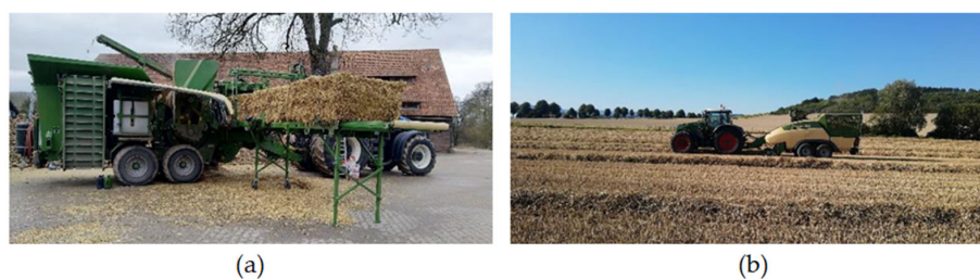
Figure 1. Industrial-scale stationary pelleting (a) and pelleting at field (b) with a mobile pelleting plant (Photos courtesy of Sören Mohrmann).
