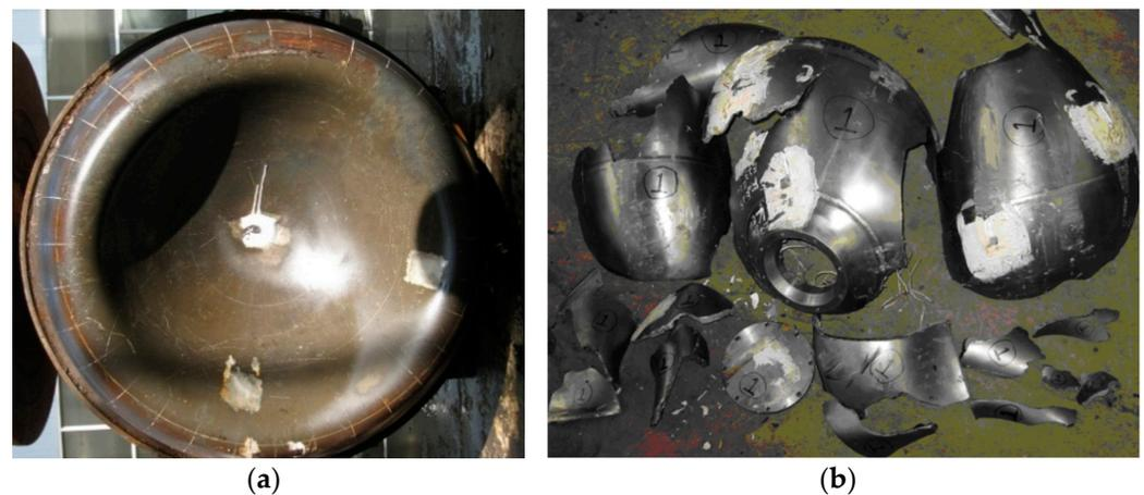
**Figure 1.** Fracture behavior of (a) high-strength steel and (b) TC4 ELI.
