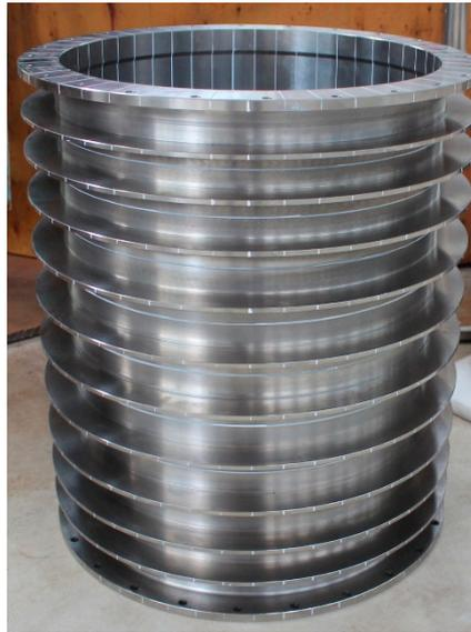
**Figure 9.** Fine-machined, ring-stiffened cylinder (TC4 ELI).
