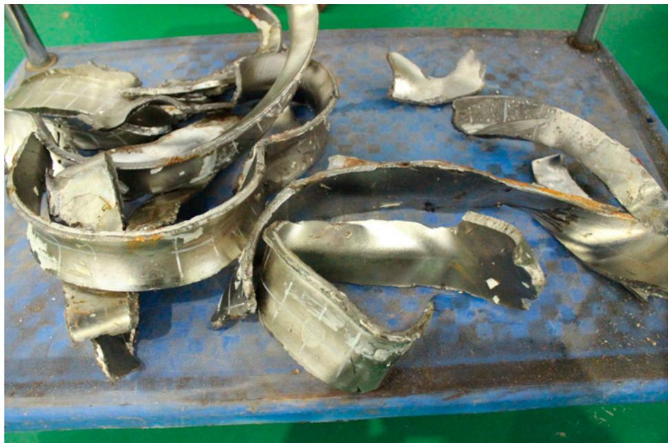
**Figure 10.** The cylinder after the external pressure experiment.
