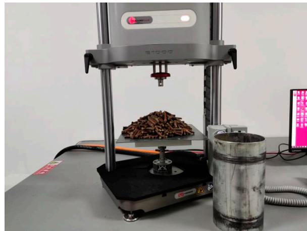
Figure 2. Cylinder-lifting method's accumulation angle-measuring instrument.
