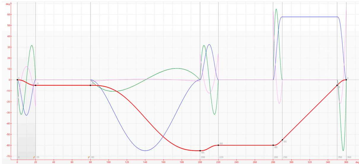
Figure 1. Electronic motion profile: red: synchronized axis position [deg], blue: synchronized axis speed [rpm], green: acceleration [rad/s 2 ], pink: synchronized axis spurt [rad/s 3 ].
