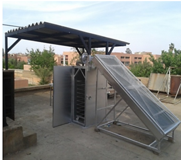
Figure 1. Convective indirect solar dryer utilized in the experiment [28].
