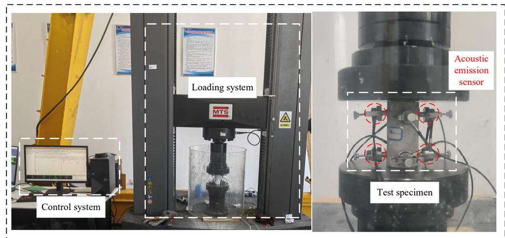
**Figure 3.** E45.605 mine rock mechanical properties test system.
