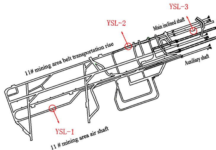
Figure 2. In-situ stress measuring point layout diagram of hollow core inclusion.
