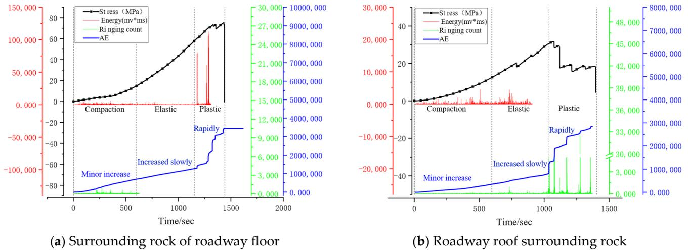
**Figure 6.** Acoustic emission ringing count and energy evolution law of No. 5 coal roof and floor rock samples.
