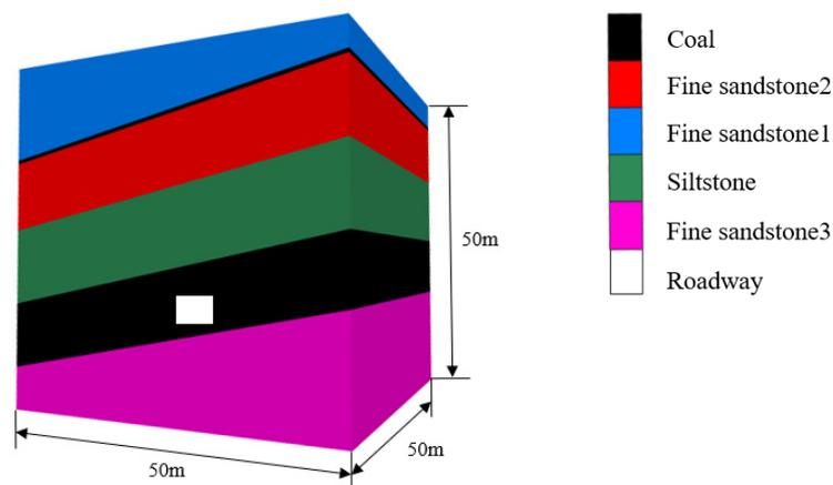
**Figure 7.** Construction of numerical calculation model of surrounding rock strata in 110,505 headentry roadway.
