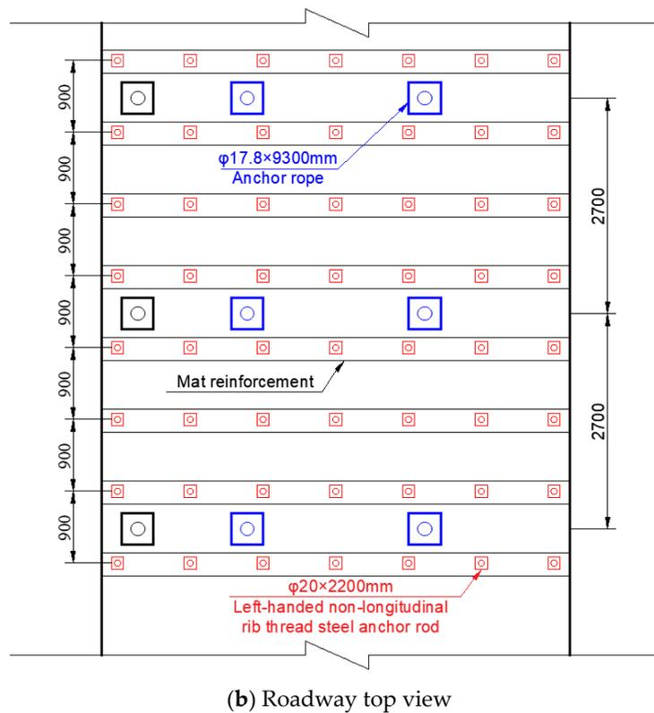
**Figure 11.** Surrounding rock control technology of the 110,505 roadway combined with an ‘asymmetric anchor net cable + pressure relief hole’.
