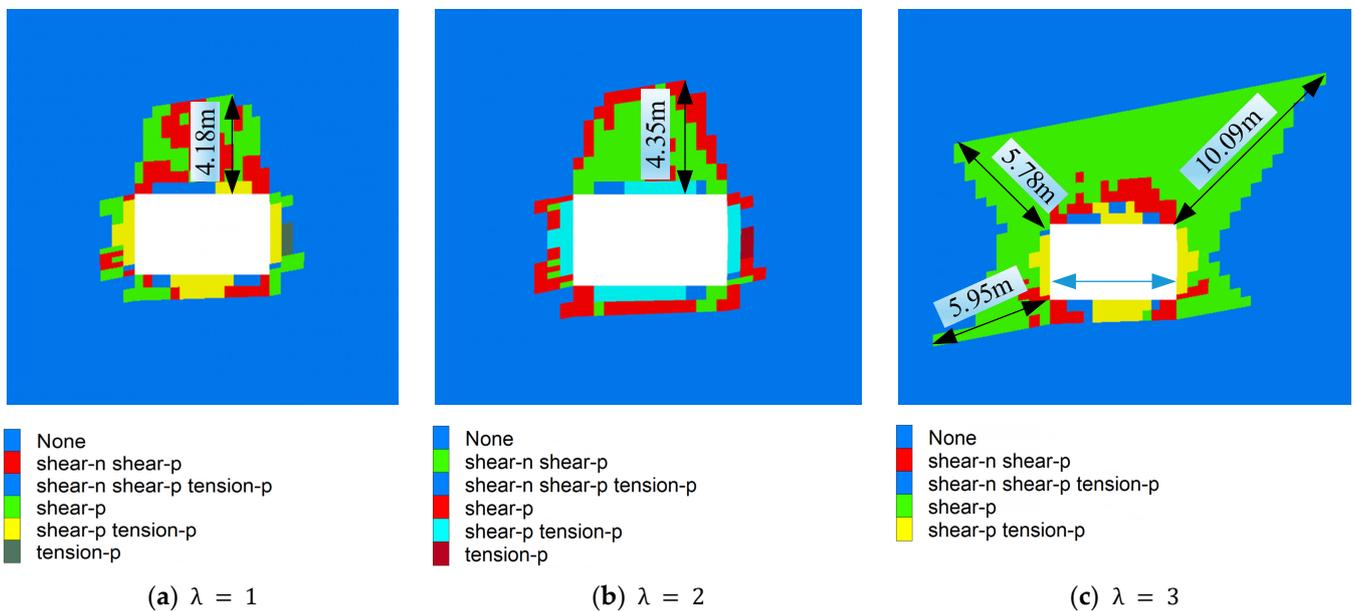
Figure 10. Cloud diagrams of plastic zone of surrounding rock of the 110,505 transportation roadway under different tectonic stress.
