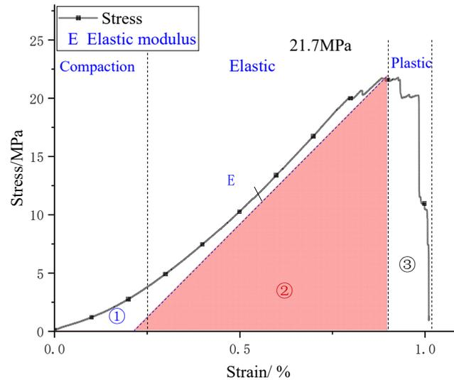
**Figure 5.** No. 5 Coal sample stress–strain curve.
