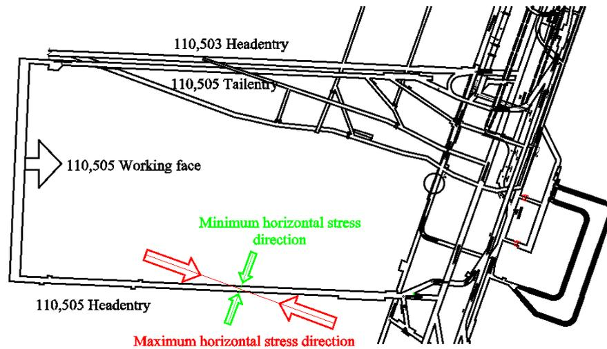
**Figure 4.** The orientation relationship between the direction of in situ stress and the 110,505 headentry.
