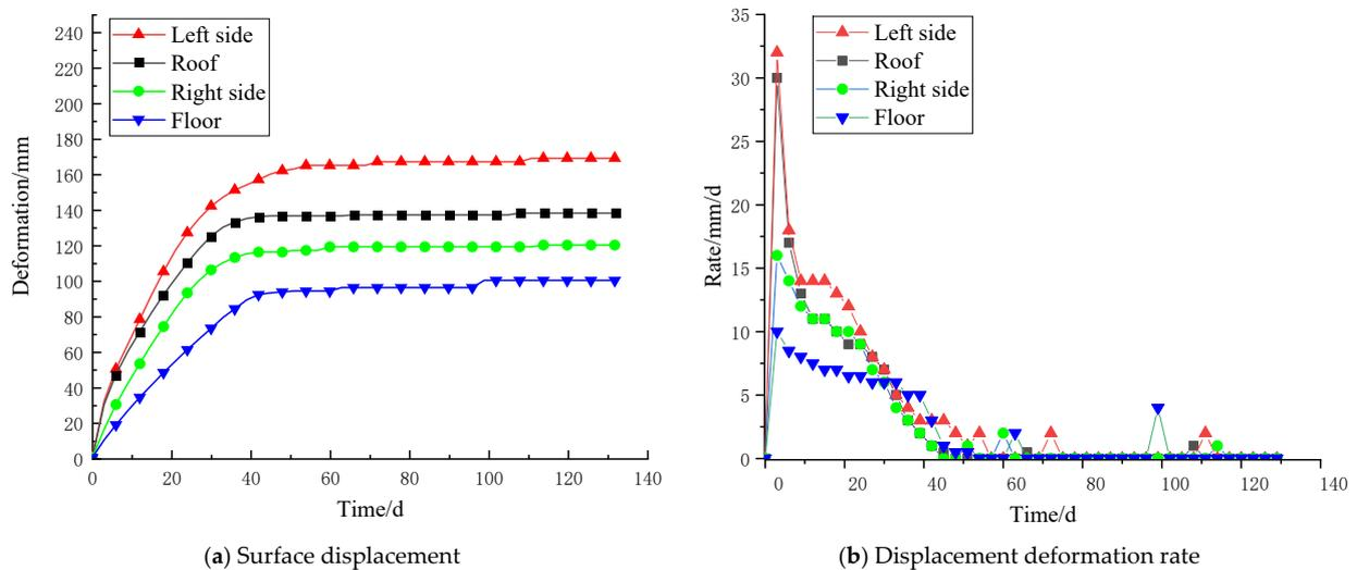
**Figure 12.** Deformation monitoring of surrounding rock of 110,505 roadway under tectonic stress.
