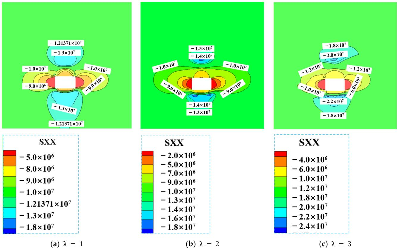
**Figure 8.** Horizontal stress nephogram of surrounding rock of 110,505 headentry under different tectonic stress.
