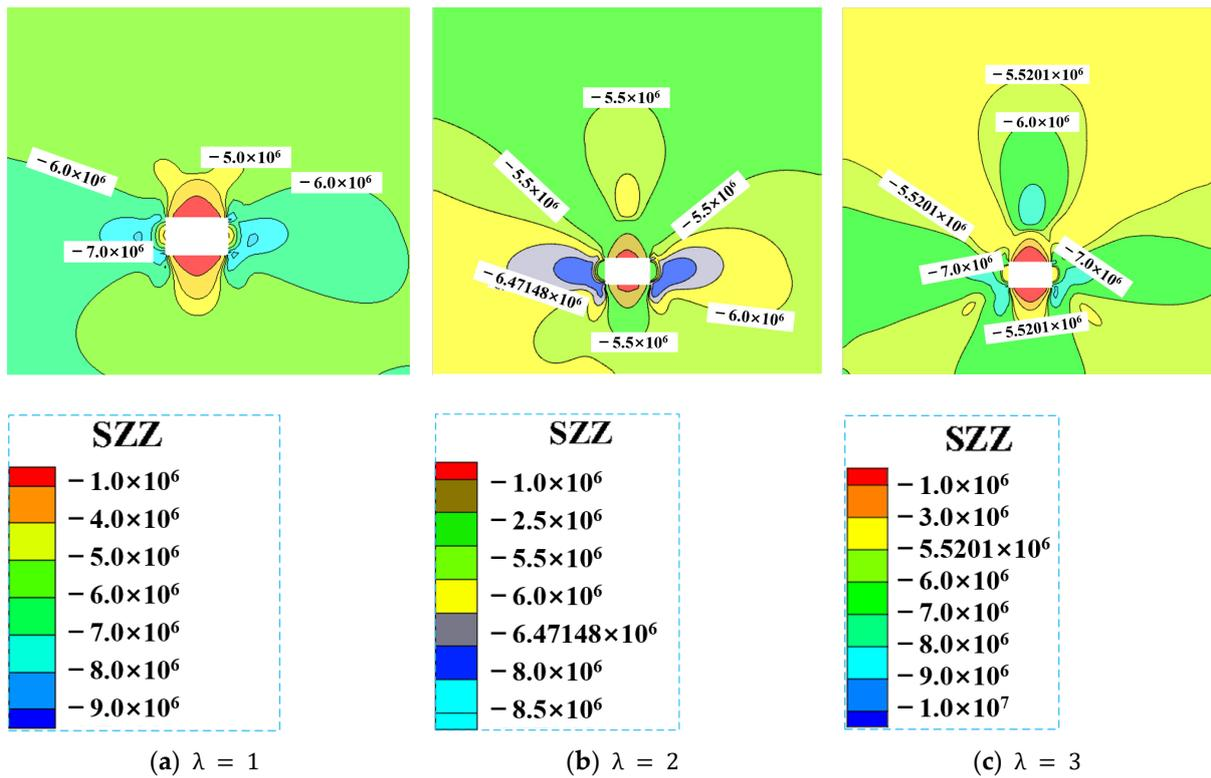
Figure 9. Vertical stress nephogram of surrounding rock of 110,505 transportation roadway under different tectonic stress.
