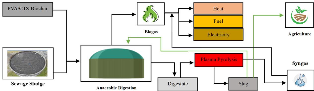
**Figure 2.** Schematic diagram of PVA/CTS-modified biochar as an additive in mesophilic anaerobic digestion (30–38 °C) treatment and co-processing with plasma pyrolysis.
