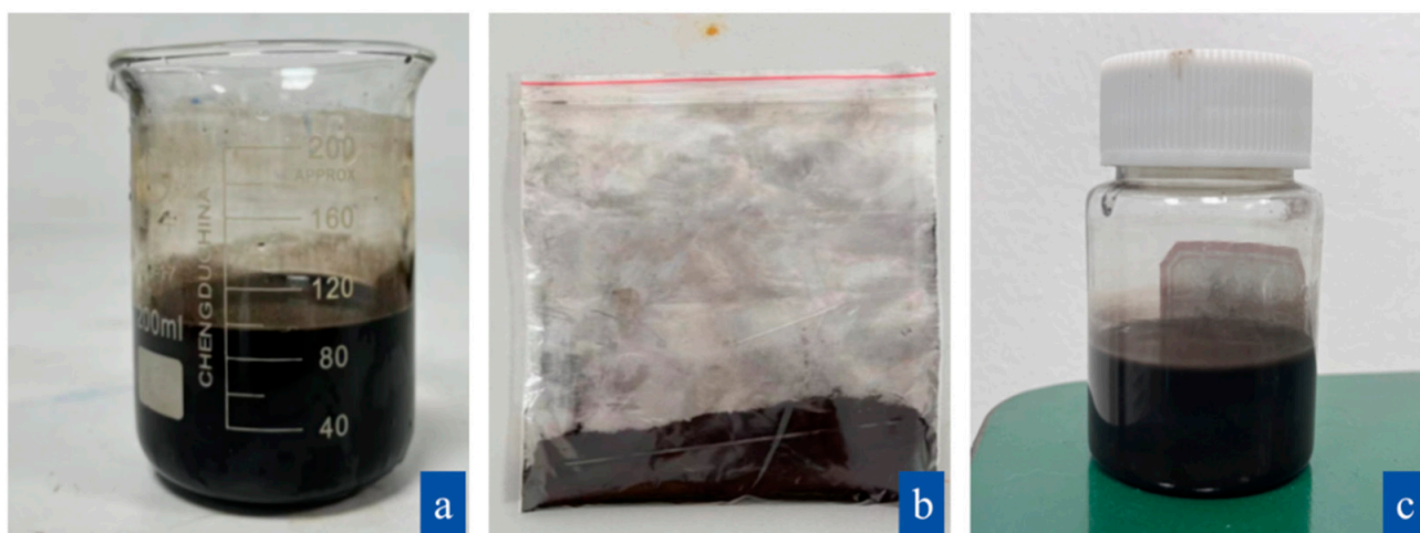
Figure 1. Samples of ferrofluid preparation process ((a) core-shell nano-magnetic particles; (b) dried nano-magnetic particles; (c) silicone-based ferrofluid).
