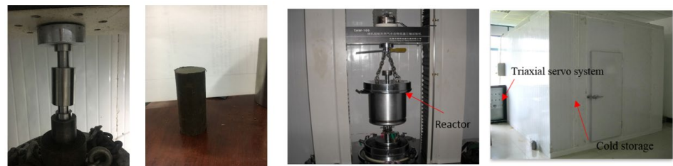
Sample pressing Artificial sample Cryogenic triaxial system Cryogenic reactor (a)
