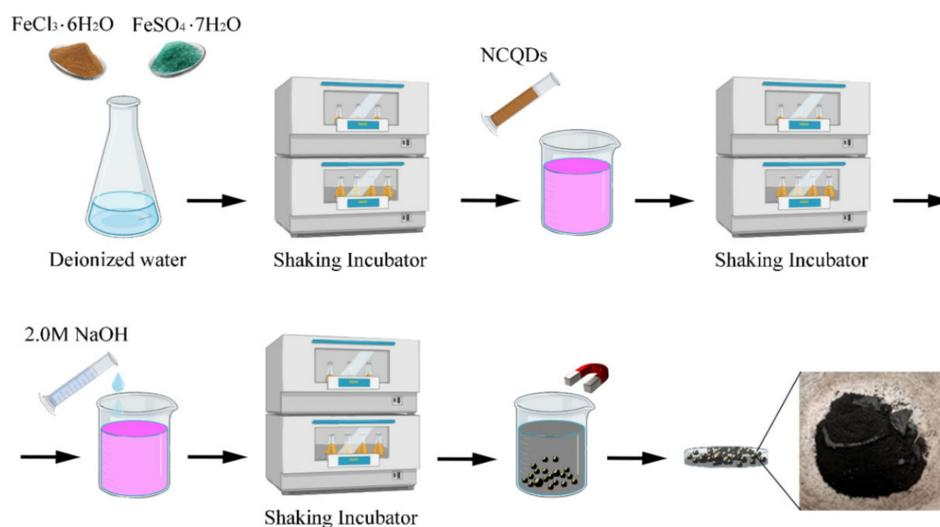
**Figure 2.** Fabrication process to obtain magnetite NCQDs in powder form.
