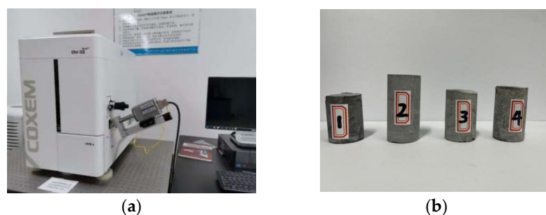
Figure 5. High-pressure mercury injection experimental instruments and samples: (a) high-pressure mercury porosimeter; (b) high-pressure mercury intrusion samples.
