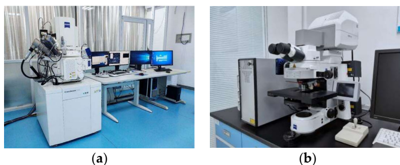
Figure 4. Experimental instruments: (a) field emission/focused ion beam scanning electron microscope; (b) laser scanning confocal microscope.
