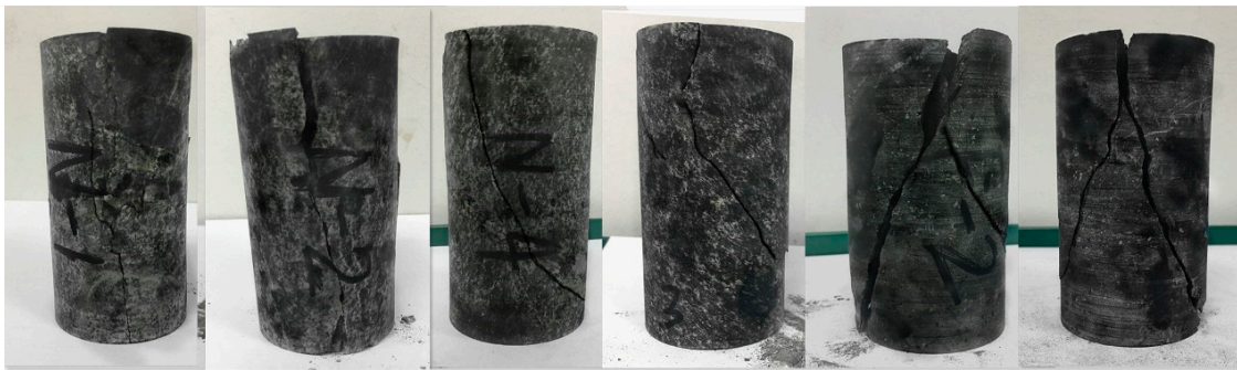
Figure 8. Images of failure in rock samples after different numbers of dry-wet cycles.
