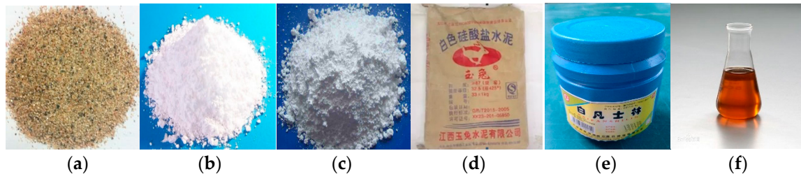
Figure 1. The raw materials of similar-material: (a) River sand; (b) Calcium carbonate; (c) Talc powder; (d) White cement; (e) Vaseline; (f) Antiwear hydraulic oil.
