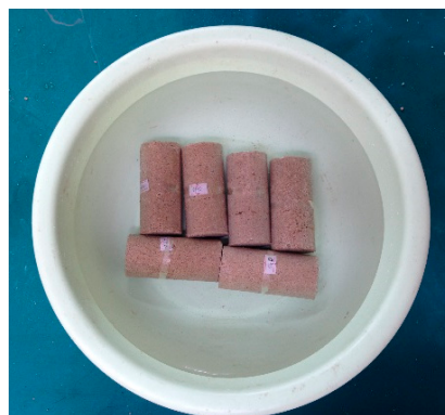
Figure 3. Testing water absorption rate.
