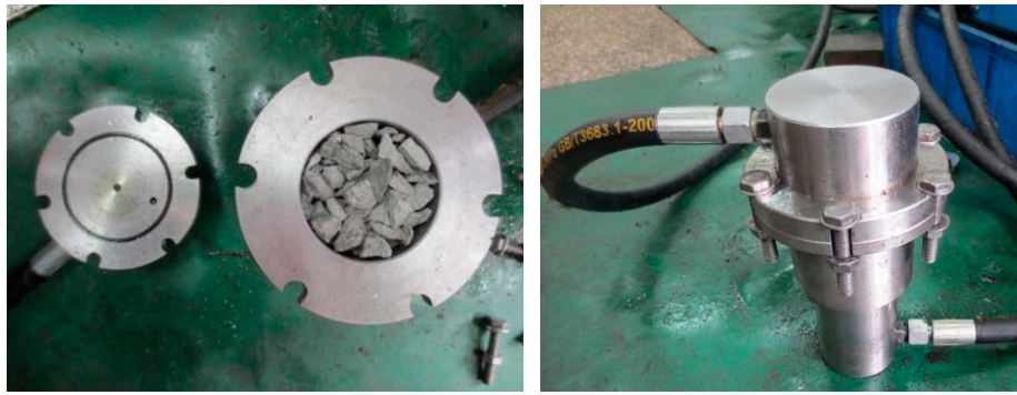
Figure 3. Filling method of the sample in the osmosis device.
