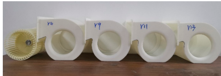
Figure 4. Impeller and volute with tongue radius r = 4 mm, 9 mm, 11 mm and 13 mm.
