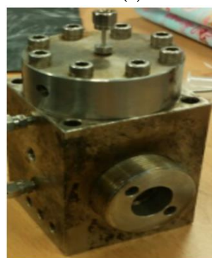
Figure 3. HPHT optical cell: (a) a schematic diagram with part details and (b) an actual equipment.
