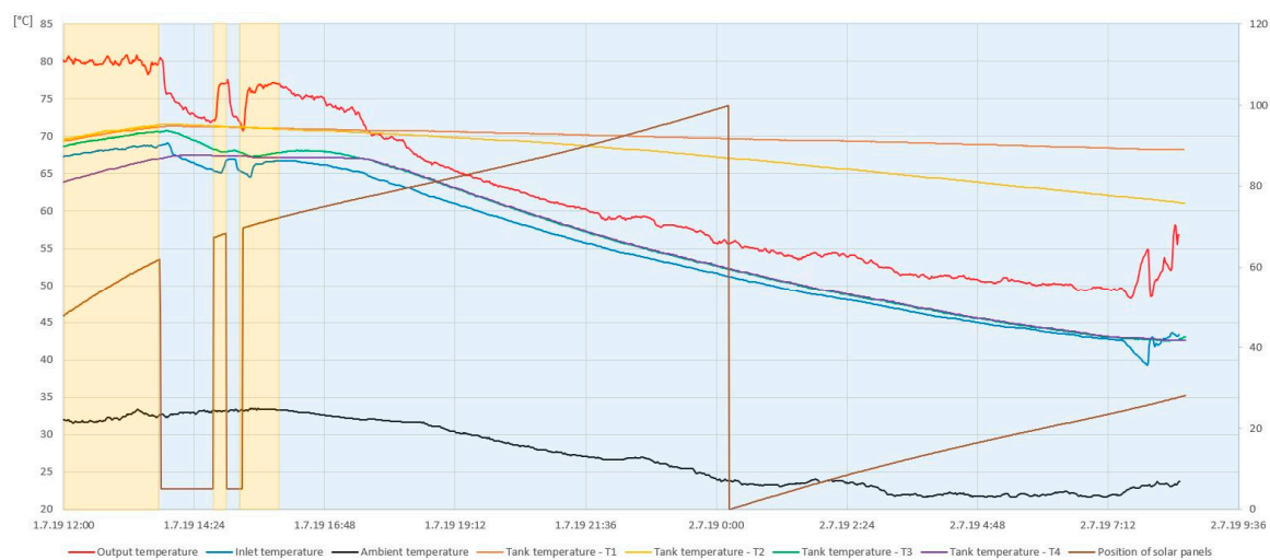
Figure 17. Influence of panel tilting on the system temperatures and liquid cooling process in the tank.
