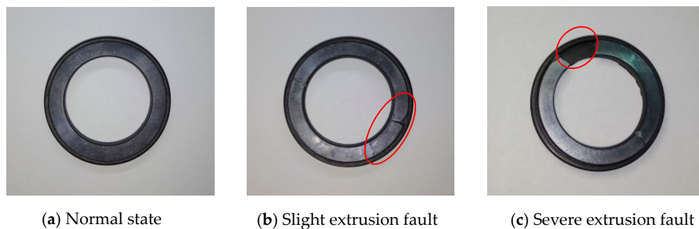
Figure 3. Rotating ring in different extrusion fault.
