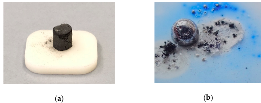
Figure 4. (a) NMC_C sample before and (b) after heating to 1600 °C in the heating microscope.
