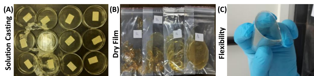
Figure 1. Digital images of the solution casting of the (A) chitosan (CH) and CH-GL films, (B) dried stored films, and (C) illustrating the flexibility of CH-GL film.
