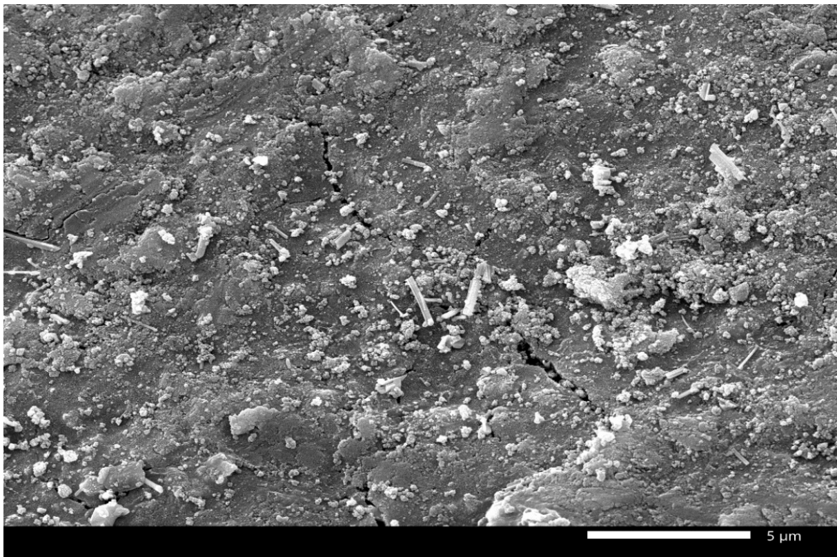
Figure 21. Photo of the spent catalyst after the blank test obtained during scanning electron microscopy (SEM).
