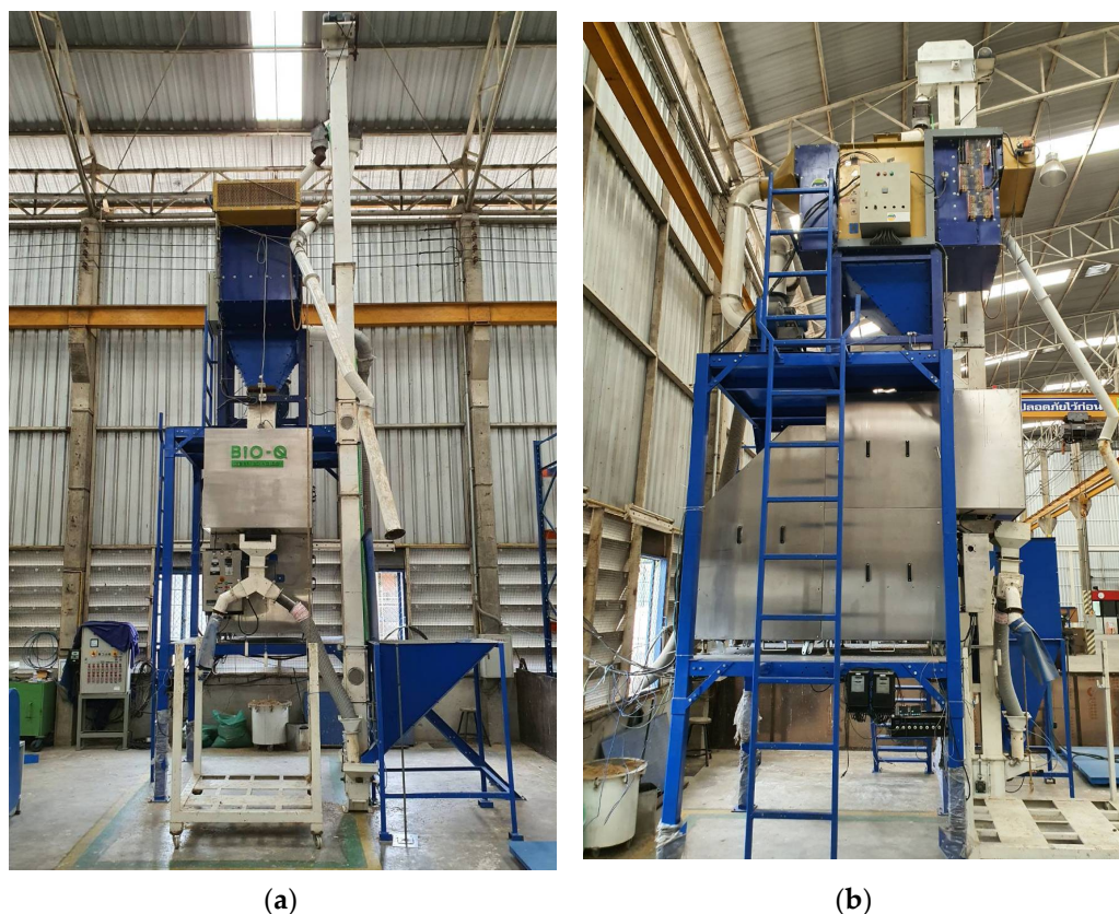
Figure 1. Prototype of the industrial-scale continuous-flow hot air dryer combined with radio frequency heating: (a) front view; (b) side view.
