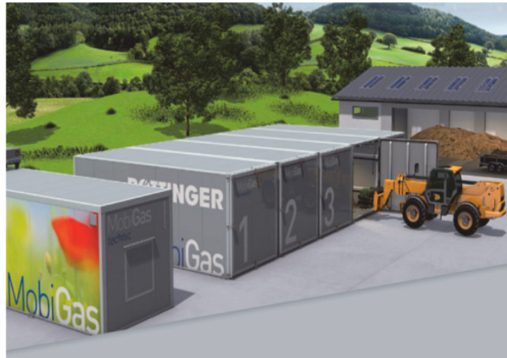
Figure 6. Simple garage type solid waste digesters [42].
