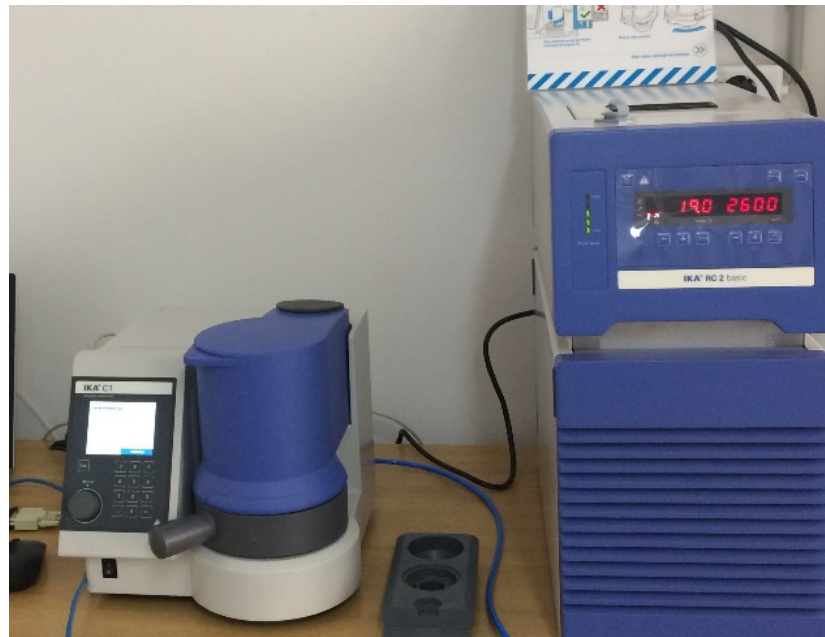
Figure 4. Calorimetric analysis for MSW sample.
