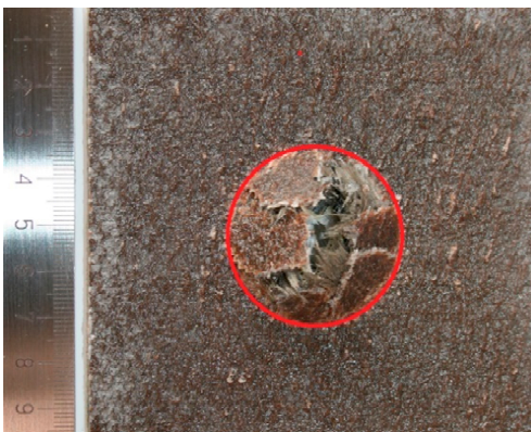
Figure 5. Photographs of impacted laminates GCABF (a), CGABF (b), CAGBF (c), MAGCBF (d), VGACBF (e), MGACBSF (f) with various damage modes.
