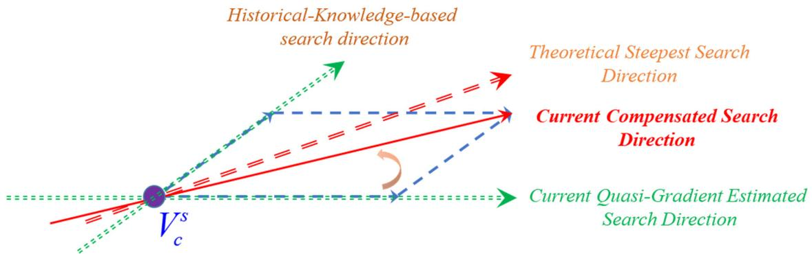
Figure 7. A sketch of the compensation mechanism.
