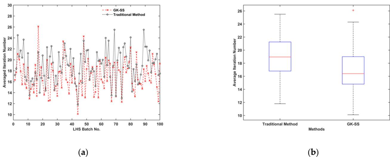
**Figure 19.** Average iteration number distribution in the test: (a) dot diagram of the average iteration numbers and (b) box plot of the averaged iteration number.
