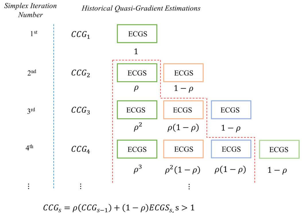
Figure 9. Historical quasi-gradient estimation storage and utilization.
