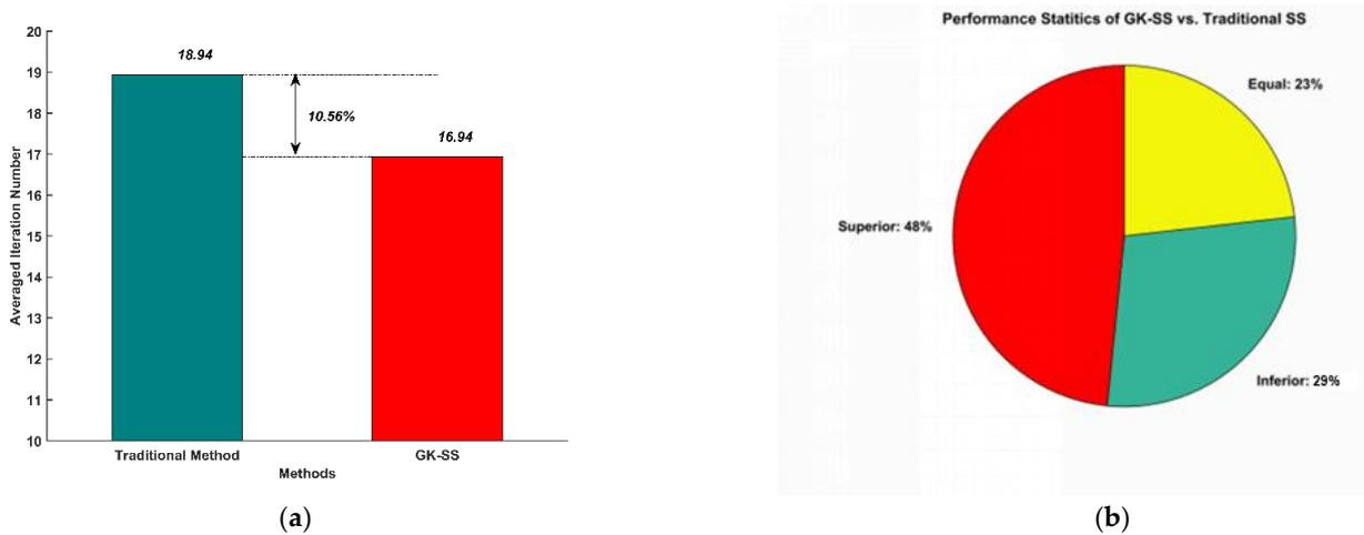
**Figure 21.** Performance evaluation of GK-SS vs. traditional simplex search method by statistics. (a) Averaged iteration number. (b) Superiority ratio by direct performance comparison.
