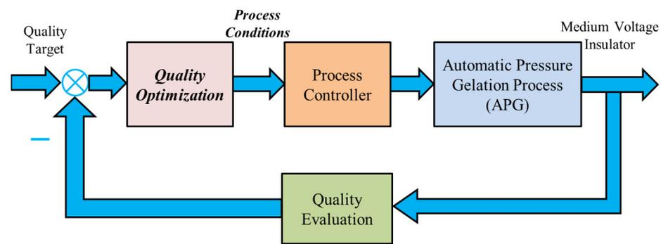
Figure 2. Quality control schematic diagram for medium voltage insulator manufacturing process. [4].
