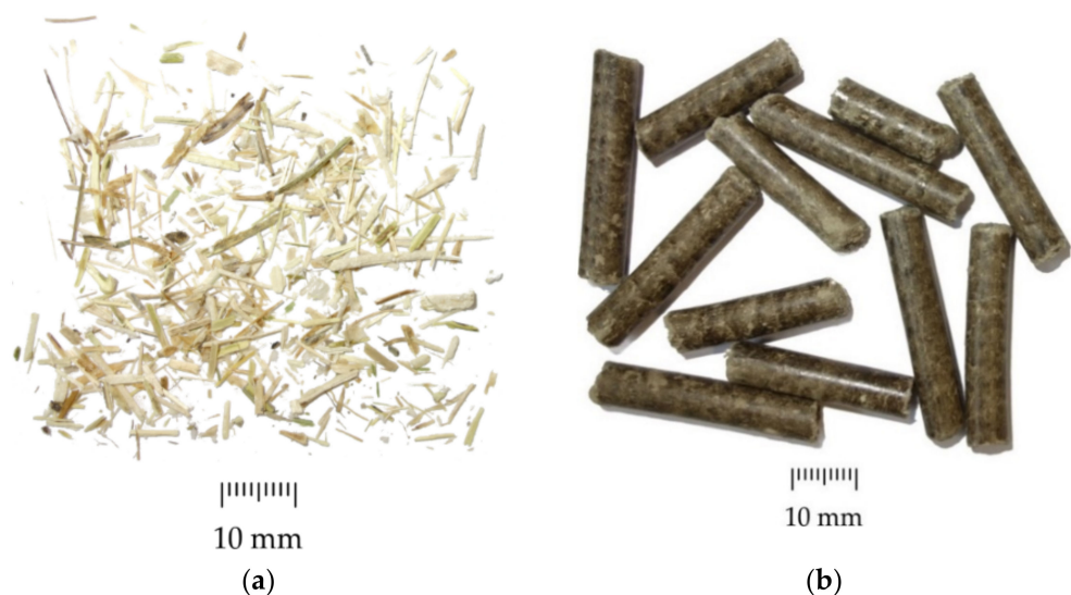
Figure 2. Biomass samples: (a) comminuted rape straw; (b) rape straw pellets.
